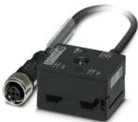
AS-Interface distributor with a high degree of protection, for a branch from two flat-ribbon conductors to a 1.0 m PUR round cable with straight M12-SPEEDCON socket
