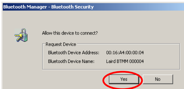
Figure 2-10: A2DP example 1 – Confirm pairing (here: Secure Simple Pairing, no PIN required)
