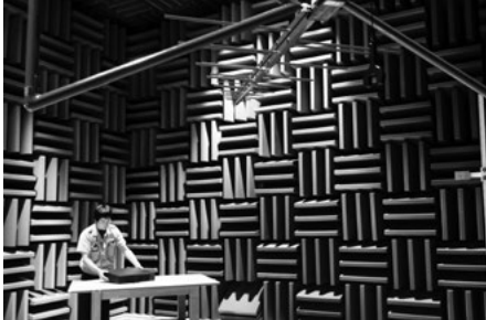
Acoustic radio wave anechoic chamber
