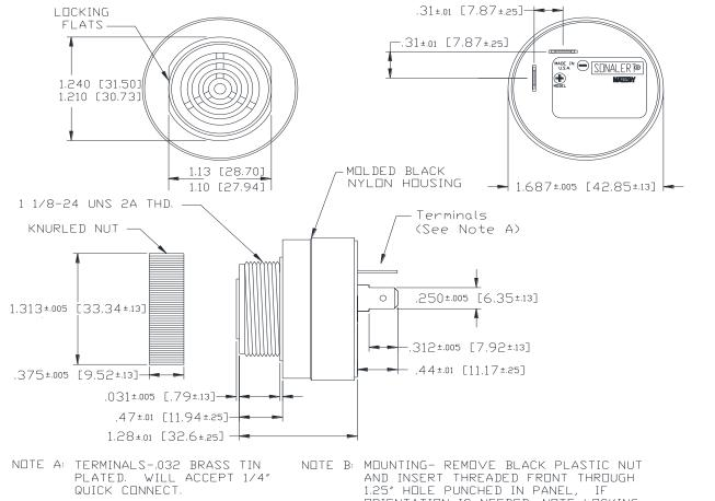
ORIENTATION IS NEEDED, NOTE LOCKING FLATS ON DRAWING. SCREW NUT BACK
