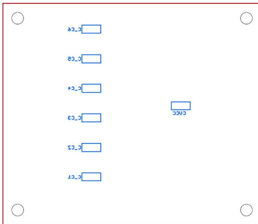
Figure 5. Bottom layer silkscreen (Top view).
