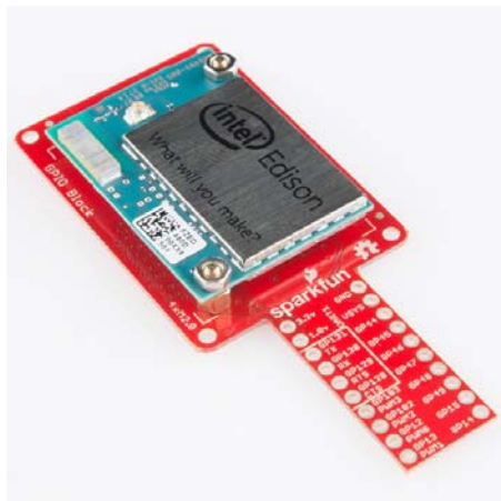
GPIO Block Installed
