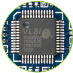
Figure 8-1: On-board VS1053 MP3 codec
