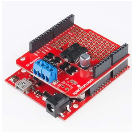
ArduMoto Shield assembled and situated on a RedBoard.
